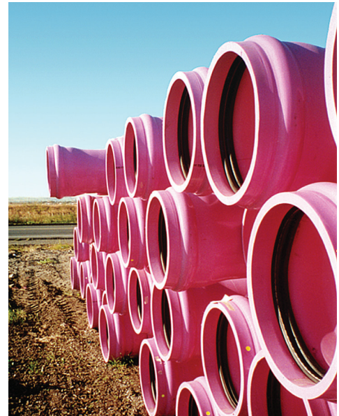
Recycled Water Pipes
