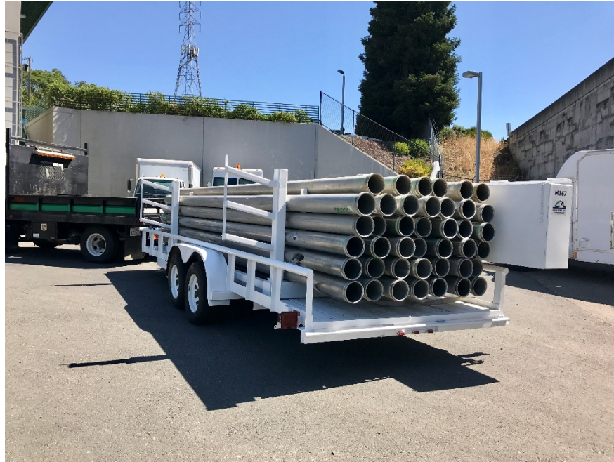
Figure 4.15 Emergency Response Pipe Trailer
