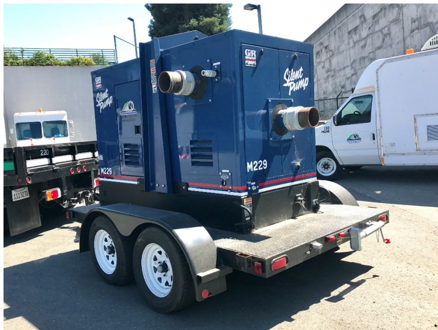
Figure 4.18 Gorman-Rupp Bypass Pump at CSO
