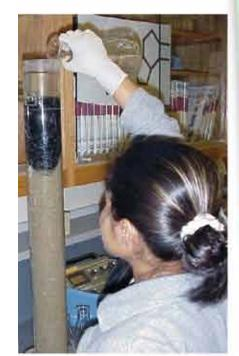
A student performs a filtration experiment during a Sewer Science class.
